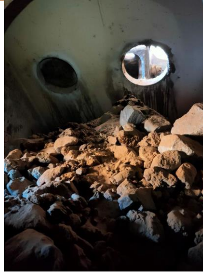
b. Clean internal car body and remove debris
