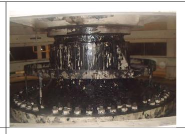
7. Upper Nut ( Under Drag Chute) - Clean away excess grease and lube build up
