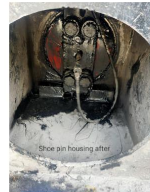
Shoe pin housing before and after bulk grease removal. Job completed.
