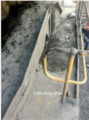
Shoes after bulk grease removal. All surface bulk grease removed. Job completed.
