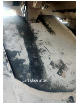
Shoe pin housing before and after bulk grease removal. Job completed.
