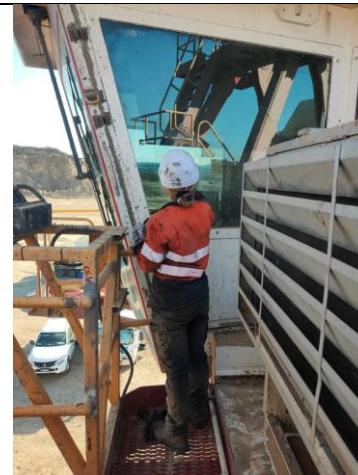
c. Clean windows and glass screen areas on operators' cabin
